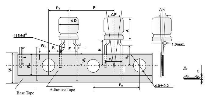
Taping dimension Unit: mm
