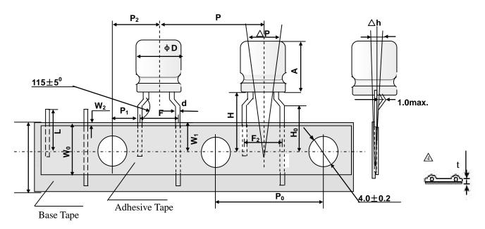
Taping dimension Unit: mm
