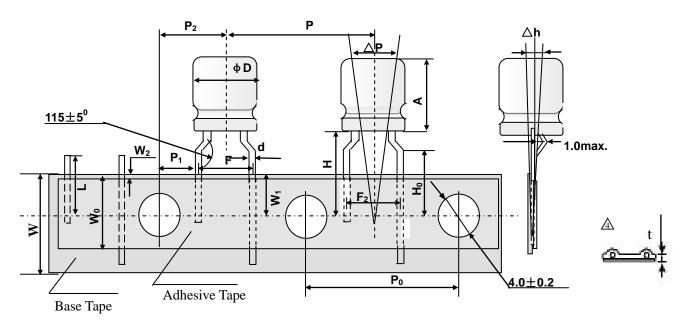
Taping dimension Unit: mm
