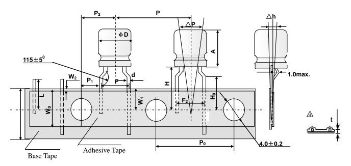
Taping dimension Unit: mm
